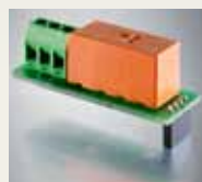
Releu conectare lumini garaj
